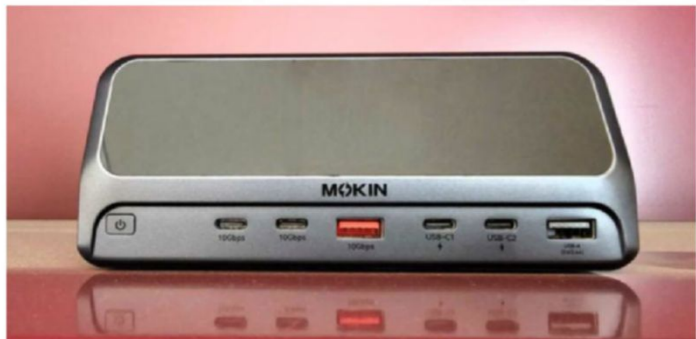
The two USB-C ports to the left, plus the centered USB-A port, all provide data but aren't designed to deliver power. The right-hand ports provide power but no data.
