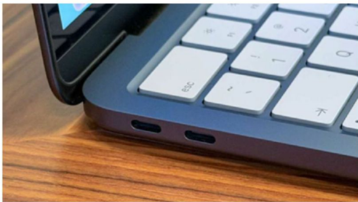
Both ports are USB-C, but the left port is faster than the right.
